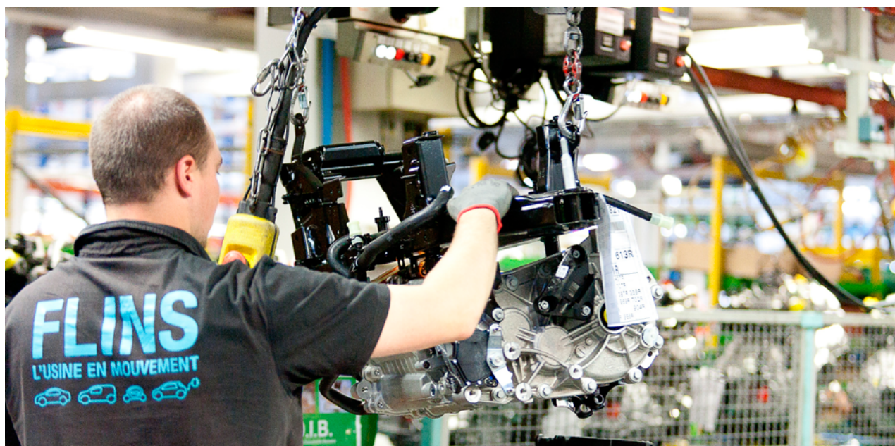
Renault Flins plant: assembly line of the ZOE powertrain
